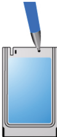
Figure 2-3: Ejecting the SIM card
