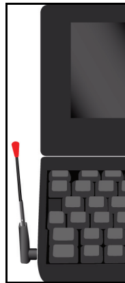
Figure 5-1: Proper positioning of the AirCard modem antenna for AirCard 850 modem / AirCard 860 modem
