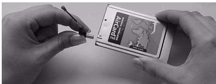
Figure 4-3: Attaching the antenna to the AirCard 750
