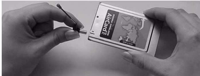
Figure 3-3: Attaching the antenna to the AirCard
