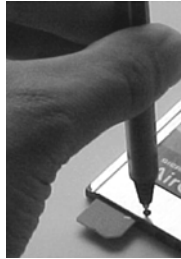
Figure 2-4: Ejecting and removing the SIM card
