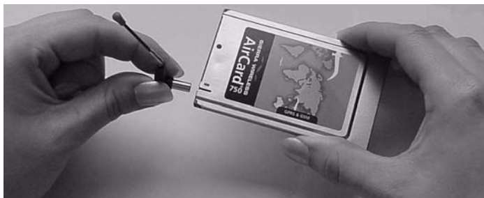
Figure 3-5: Attaching the antenna to the AirCard
