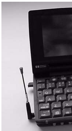
Figure 6-1: Proper positioning of the AirCard antenna
