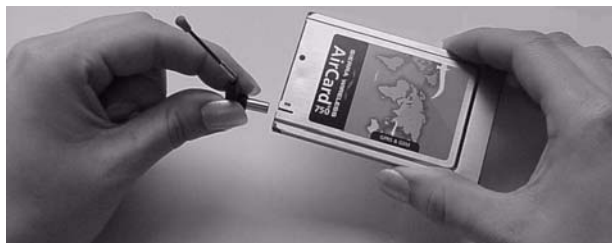
Figure 3-1: Attaching the antenna to the AirCard
