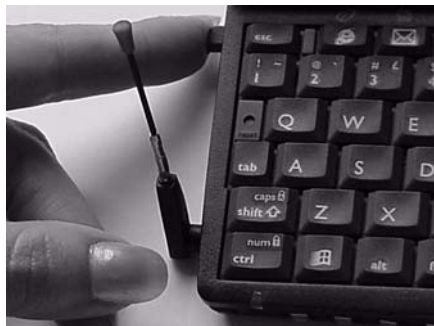
Figure 6-4: Ejecting the AirCard from its slot
