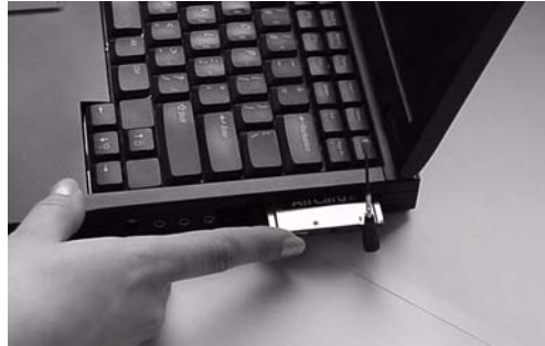
Figure 3-2: Inserting the AirCard
