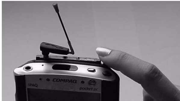
Figure 6-3: Removing the AirCard from its slot (Pocket PC)
