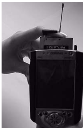
Figure 4-2: Inserting the AirCard into a Pocket PC
